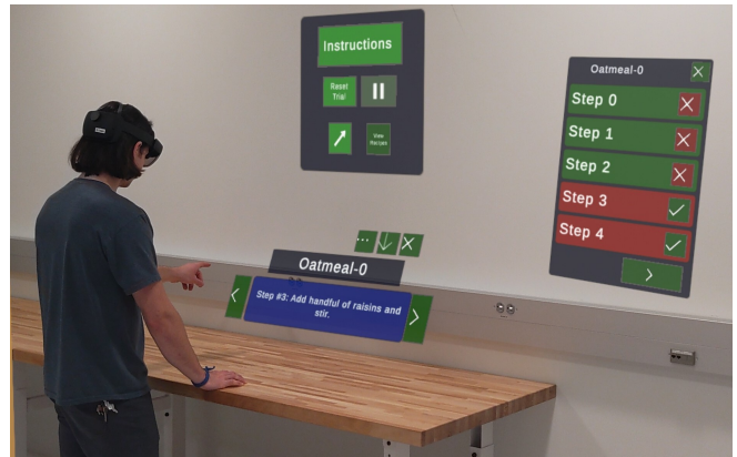
Figure 1: A user interacting with the UI. Included elements are the main menu (top), instruction panel (bottom), and task list view (right).
